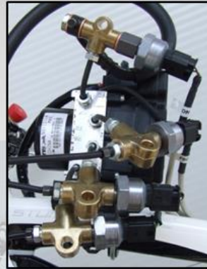
HECU and Pressure Sensors
