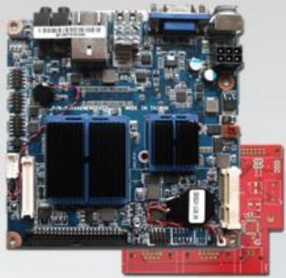
Controller Computer and A/D Converter
